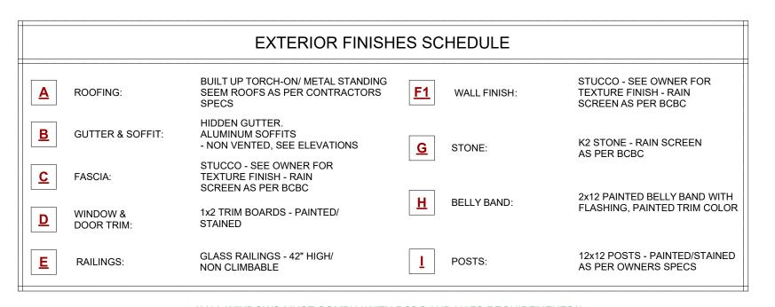
\*\*ALL WINDOWS MUST COMPLY WITH BCBC AND NAFS REQUIREMENTS\*\* MUST BE CLEARLY LABELED ON ALL WINDOW UNITS UPON INSTALLATION FOR INSPECTION. -ONE EXTERIOR DOOR IS PERMITTED TO HAVE A HIGHER U-VALUE OF 2.6, ALL OTHERS MUST BE LOWER. -GARAGE VEHICULAR DOORS MUST BE MINIMUM NOMINAL RSI OF 1.1
